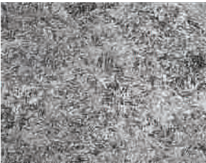
Figure 2: Acceptable microstructure after welding. (100X) (1)
