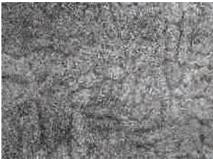
Figure 1: Acceptable microstructure of castings (100X) (1)
